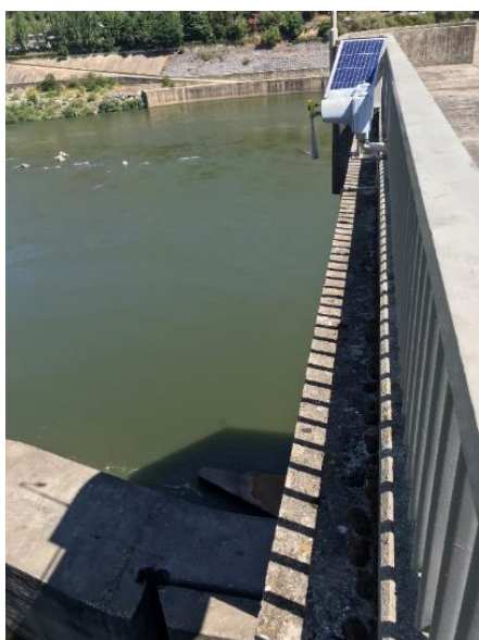
Figure 2 - Limnimeter and water velocity sensor at Regua bridge
